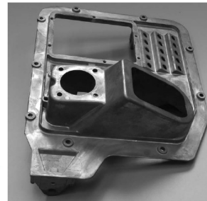
FIGURE 11.16 A large die casting measuring about 400 mm diagonally for a truck cab floor. (Courtesy of George E. Kane Manufacturing Technology Laboratory, Lehigh University)
