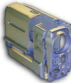
The Sharp VL-PD1 video camera features a thixomolded magnesium thin wall (<1.0 mm) external case.
